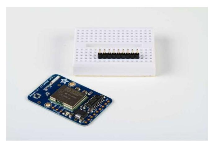
Set the breakout board over the pins, and carefully solder each pin (see our Guide To Excellent Soldering (http://adafru.it/aTk) for instructions and tips on getting the best results).
