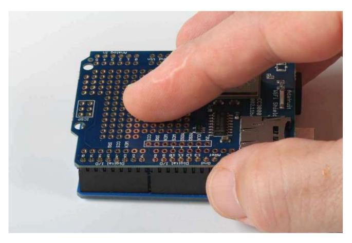
Place the shield over the pins, and carefully solder each one in place (see our Guide To Excellent Soldering (http://adafru.it/aTk) for instructions and tips on getting the best results).
