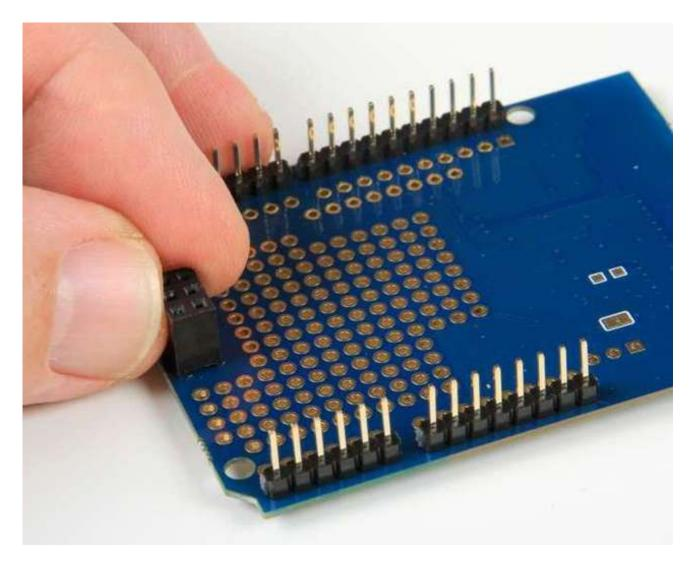
The shield also comes with a 2X3 pin female header socket. This will plug into the 2X3 ICSP pin header on your Arduino, to bring SPI up to the shield. This allows you to use the shield with an Arduino Mega or Leonardo without having to cut traces or solder jumper wires for SPI.
