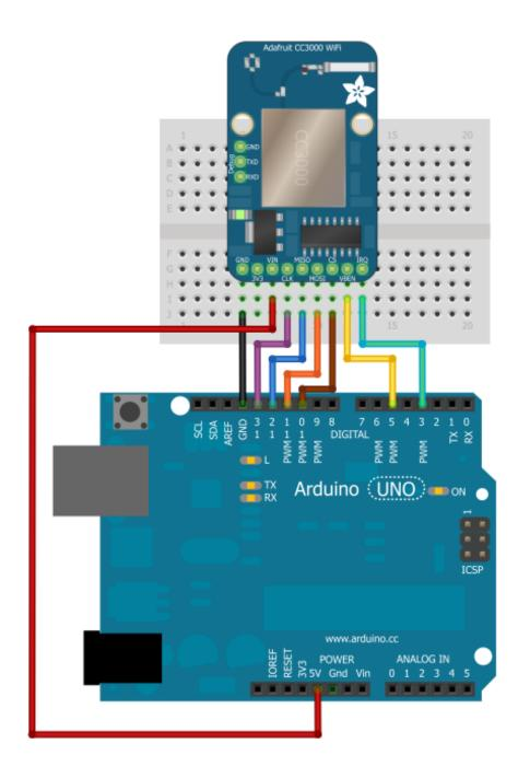
3.3v is an output from the breakout board's voltage regulator - we won't be connecting anything to it in this tutorial.
